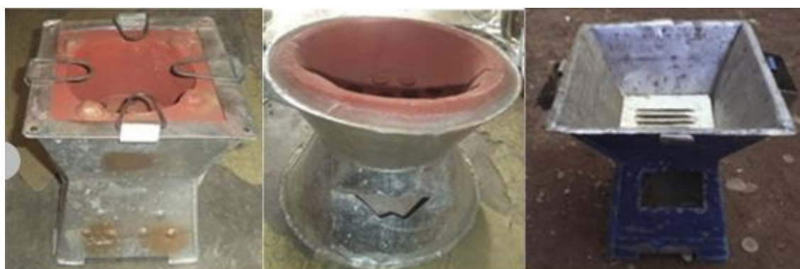
Left side – Mirchaye (7.5 L water / 478 g of charcoal / day) Middle – Laketch (7.5 L water / 536 g of charcoal/ day) Right side - tradition metal cookstove (7.5 L water / 700 g of charcoal/ day)
