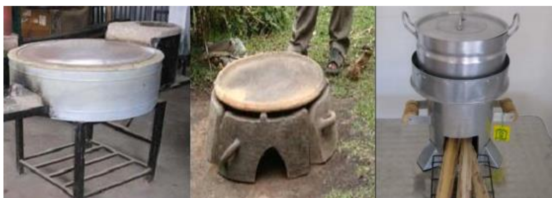
Left side - Mirt (Tier 0: Fuel use: 393 g/kg) Middle - Gonzye (Tier 0: Fuel use: 617 g/kg) Right side - biomass pot-size cookstove named Tikikil (Tier 2: Thermal efficiency: 26%)
