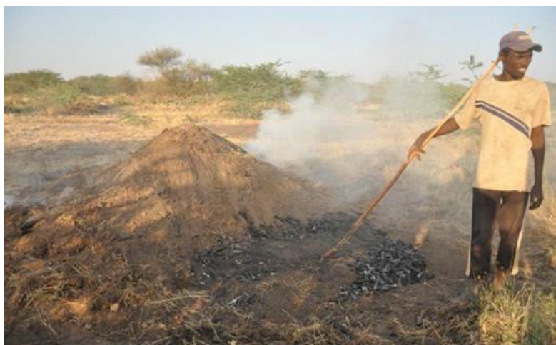
Figure 3.5. Earth-mound charcoal production
